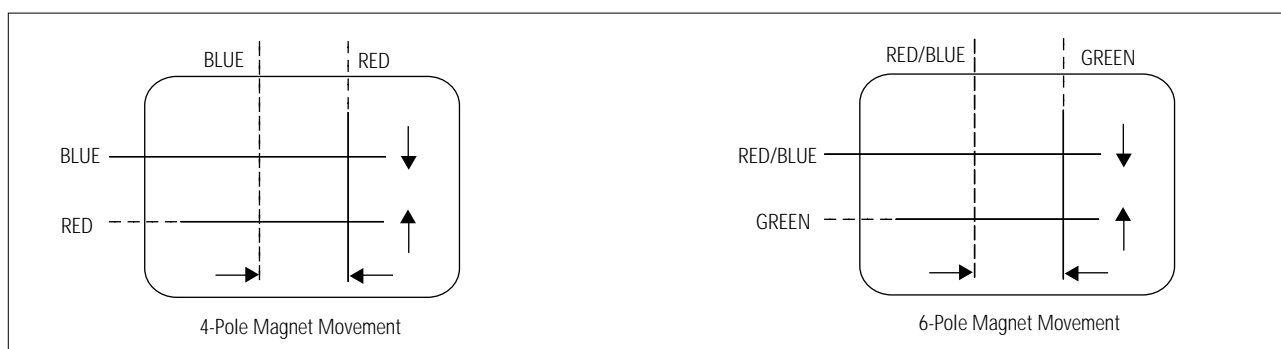
Fig. 4-5 Center Convergence Adjustment
